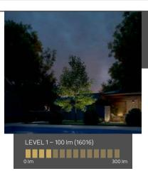
When lighting a young tree, we recommend using a cross-lighting technique with two VLO 3000K Small 35 Degree Floodlights (16016), as shown above
